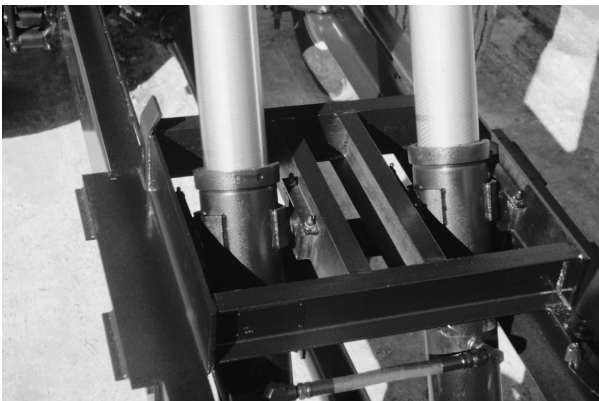
Heavy 3/8" Steel Plate Frame With Cylinders Inside Truck Frame For Superior Stability
