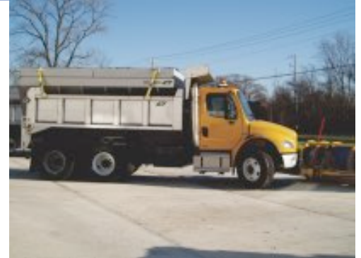
14' WXL body & E/AC2420 Spreader in 304 Stainless Steel
